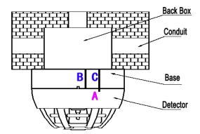
Step 1: Align Sign A of the detector body with Sign B of the base.
