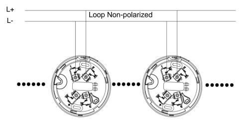
4) The alert base and detector shall be installed as the following diagram:
